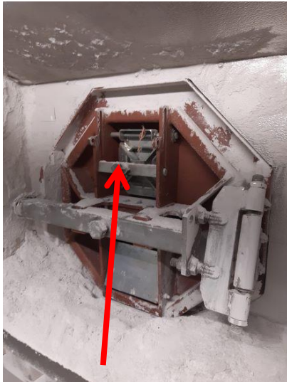
Small Inspection Opening
